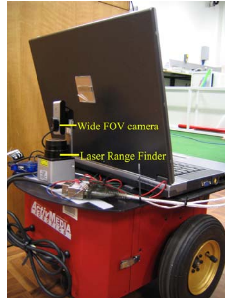
Figure 1 Wide FOV camera and laser range finder mounted on Pioneer robot
