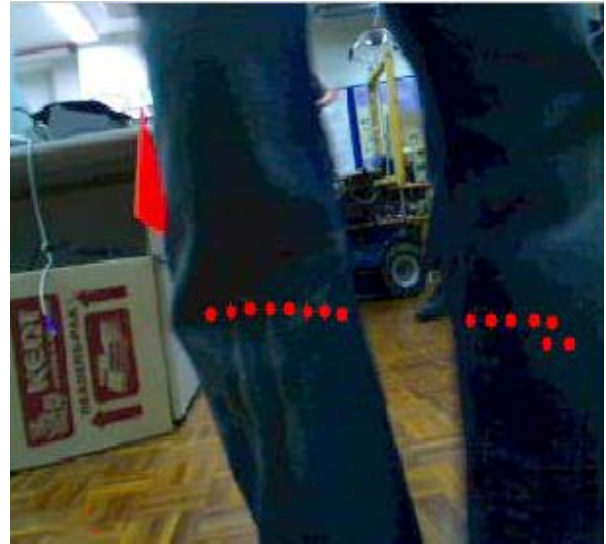
Figure 5 Laser leg segments projected onto image
