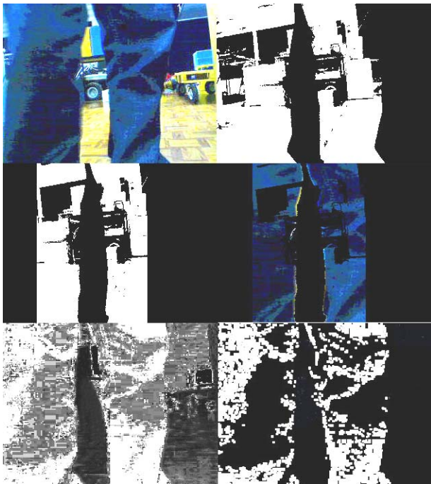
Figure 6 Steps in buildup of colour model. Left to right raster from top left: Original image, binary foreground image, binary foreground image anded with laser mask, colour samples used for modelling ,colour probability image, backprojected image
